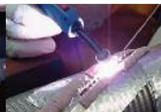
TIG repair of a broaching tool with UTP A 696
