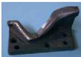
Changes of pattern of cutting jaws made from I.2382 with UTP 73 G 2
