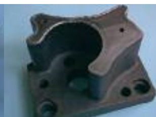
Edge coating on cutting jaws made from I.3343 with UTP 690
